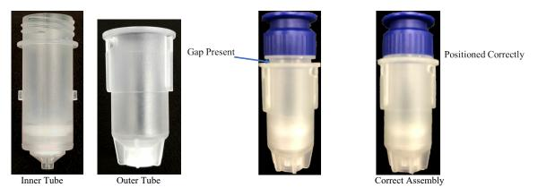
**Note**: Proper positioning of the SpermX inner tube into the lower position is critical for proper retention of solution and digestion. Incorrect positioning of the SpermX inner tube, not seated all the way to the bottom (gap present), will result in loss of solution, inefficient digestion and poor recoveries!
